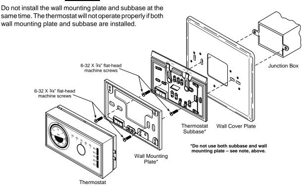
Figure 4. Mounting 1F7X quartz clock thermostat to horizontal junction box
